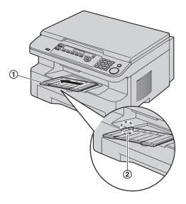
2. Snap the extender (③) into the unit by pushing down the right side of the extender.
